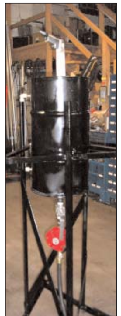
One of the CU Buff Buses (above), soon to be petroleum-free. A potassium methoxide reactor (right) is used to create fuel from vegetable oil in the biodiesel refining process.
